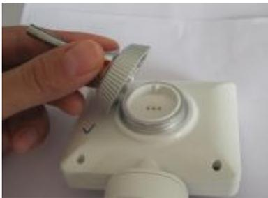
Turn the screw cap to the right until it has been tighten
